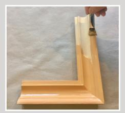
All surfaces should be smooth, clean, and free from dirt, dust, and grease. Prime surface if necessary and let dry. In this example, I've primed the wood sample with shellac.
